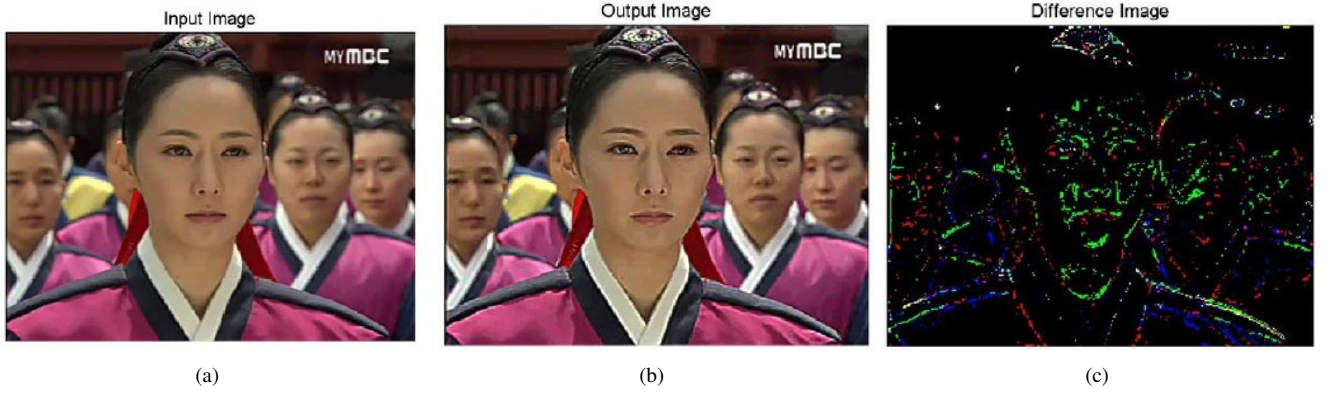
Fig. 3. Sharpness enhancement of sample frames of video clip “Human”: (a) Input image, (b) Output image, (c) Difference image.
