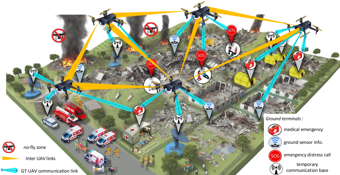
Fig. 1: Illustration of a UAV swarm providing support to various ground terminals in a disaster-stricken area.
