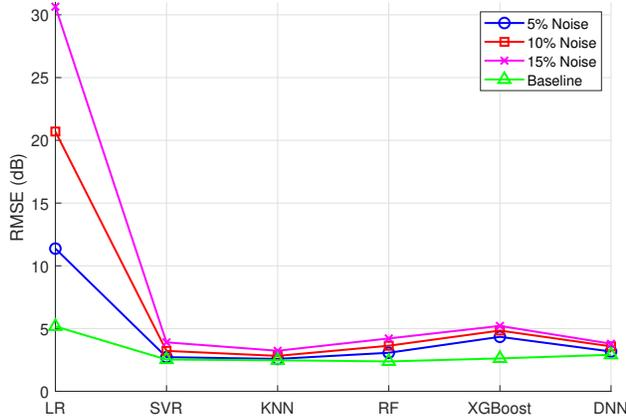
FIGURE 7: Performance comparison with noisy input features.
